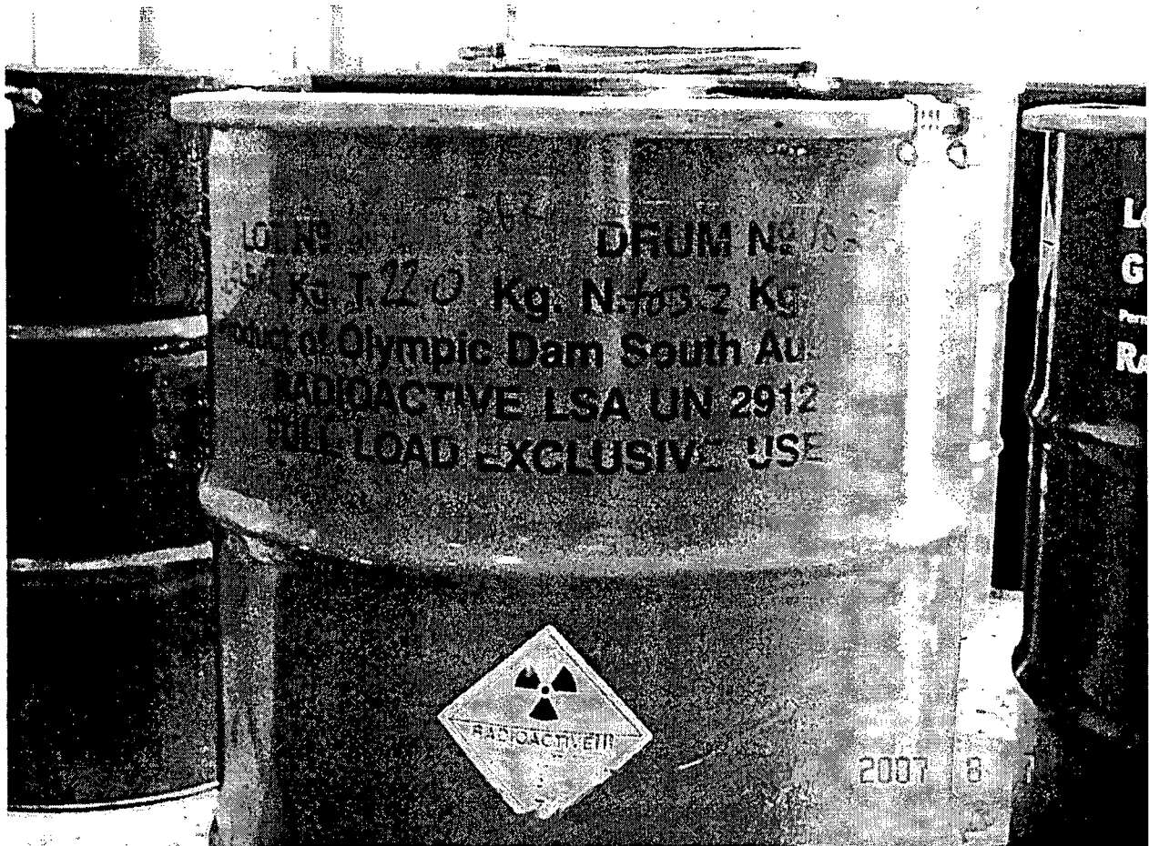
Figure 2.4-6. Labeled and Placarded 208-L [55-gal] Drum Used for Packaging and Shipping Yellowcake
