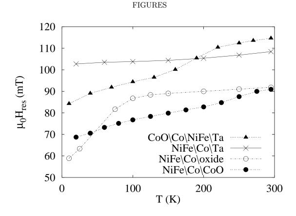
FIG. 1. Average in-plane ferromagnetic resonance fields as a function of temperature. For films coupled to CoO or allowed to oxidize, changes in slope relative to the Ta-capped control sample (NiFe\Co\Ta) indicate the onset of rotatable anisotropy.
