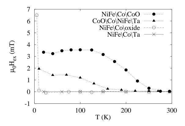
FIG. 3. Unidirectional exchange bias field measured by FMR as a function of temperature in thin magnetic films coupled to CoO. The lowest temperature data point for the NiFe\Co\oxide sample is measured by SQUID magnetometry.
