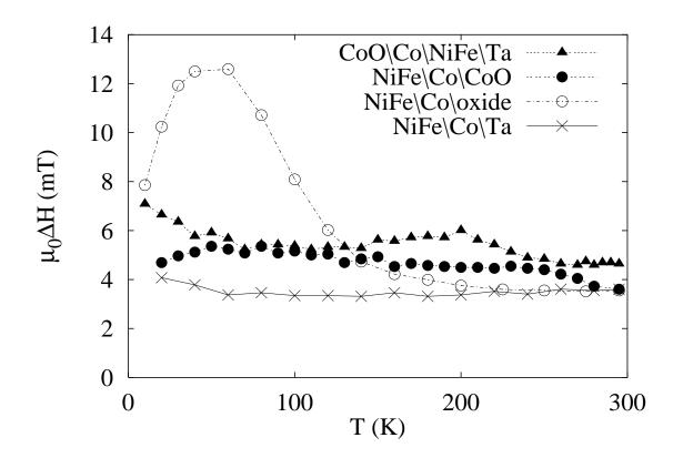
FIG. 2. FMR linewidth as a function of temperature in thin magnetic films. Peaks in the linewidth are characteristic of relaxation processes with rates comparable to the inverse precession time.
