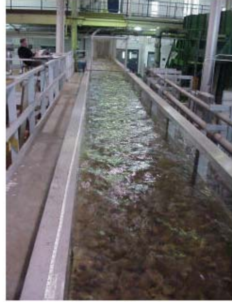
Figure 5 - View looking downstream in the 3 ft wide by 60 ft long by 1.5 ft deep adjustable slope flume.
