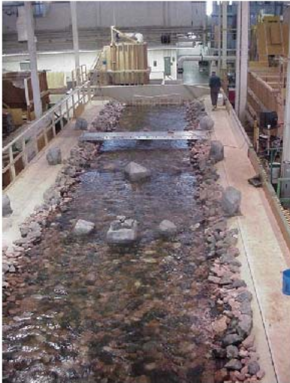
Figure 26 - View looking downstream at rock lined fishway channel with boulder weirs.
