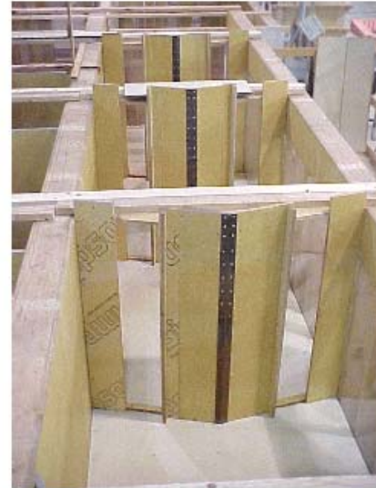
View of dual-vertical slot style baffle fishway looking downstream.
