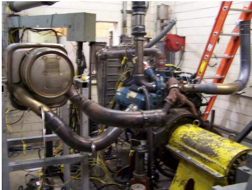
Figure 1. Engine shown installed in emissions test cell with PUREM PMF GreenTec 1004205.00.0 shown left of engine.
