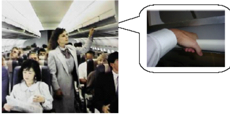
Figure 3 Handrails under the overhead stowage on MD90
