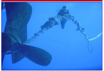
During the pre-dawn hours of the 11<sup>th</sup> of May, NOAA Ship HI'IALAKAI propellers became entangled by a 3 inch towing hawser with a 1/2inch diameter wire towing bridle woven into one end. It was discovered through the rhythmic thumping on the hull as the screws turned. A dive was organized to remove the debris from our props before it would cause serious damage.
