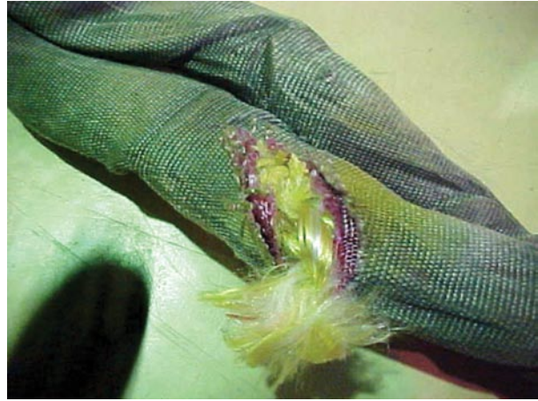
Figure 1-1. Synthetic web sling damaged by sharp edges of steel lifting attachment
