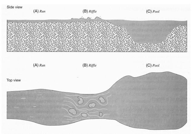
Diagram of the three main geomorphic channel units. (A) Run—A slow moving, relatively shallow body of water with moderately low velocities and little or no surface turbulence; (B) Riffle—A part of the stream where the water flows swiftly over completely or partially submerged obstructions to produce surface agitation; (C) Pool—A part of the stream with reduced velocity, commonly with deeper water than surrounding areas (modified from Bisson and others, 1982).
