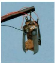
**FIGURE 2**: 4-finger EAP gripper lifting a rock.
