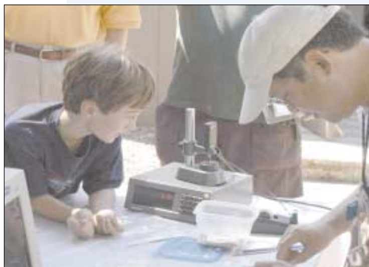
A guest waits his turn as David Urabe of MMED/MoM Group mounts a visitor's hair sample to be tensile strength tested.
