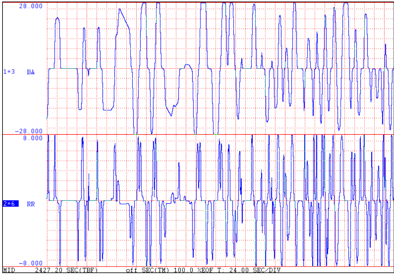
Figure E-3. Plots of Bank Angle and Roll Rate for the Last Third of the Worst-Case Flight
