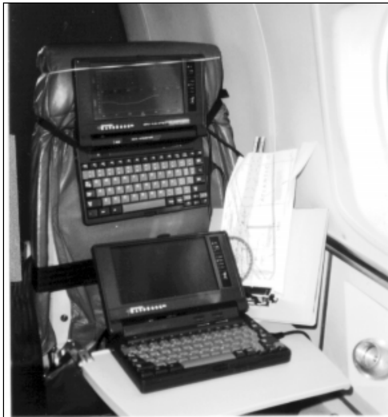
Figure 2-9. Notebook Computers Used for Data Acquisition and Generation of the Cockpit Display
