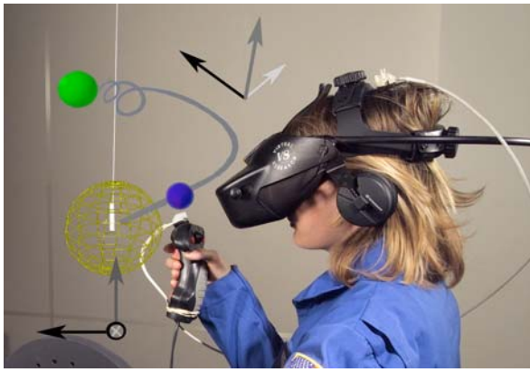
Figure 1. Schematic illustration of the subject's task. The subject moved a 3D cursor shown as virtual ball just above the tracked handle. The cursor was moved from a starting point within the larger wire-frame sphere just at the end of the hanging white plumb bob to contact a the medium-sized ball-like target shown in the upper right. The curved path shows a typical corkscrew structure that participants tended to exhibit when experiencing a coordinate rotation like that illustrated between the coordinate frame in the lower left and that in the upper center of the figure. The plumb bob could be felt to find the initial starting point of the motion. Neither the coordinate frame icons nor the path trace were visible to the subject. The starting sphere did not remain visible once the targeting motion was started.
