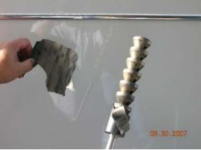
I had an experience several years ago with this type of suppressor but with a much less drastic ending. After firing a .17 Cal. rifle, the rifle/suppressor hissed for about 4 seconds before finishing with a mild "whump." The rifle and suppressor had been cleaned about a week prior to this incident but had not been fired since the cleaning. It was believe that some cleaning solution remained, which caught on fire.
