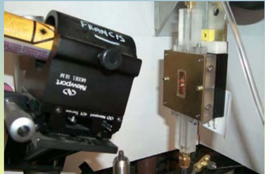
New In-situ optical device for measuring scale University of Minnesota
