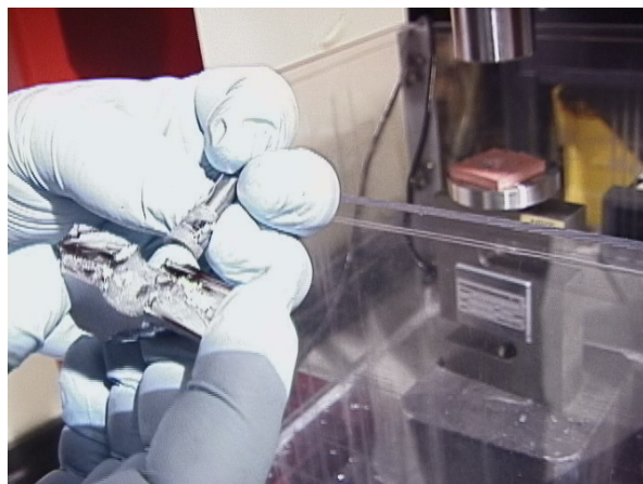
Post Rupture Reveals Excellent Frit Adhesion to Insert
