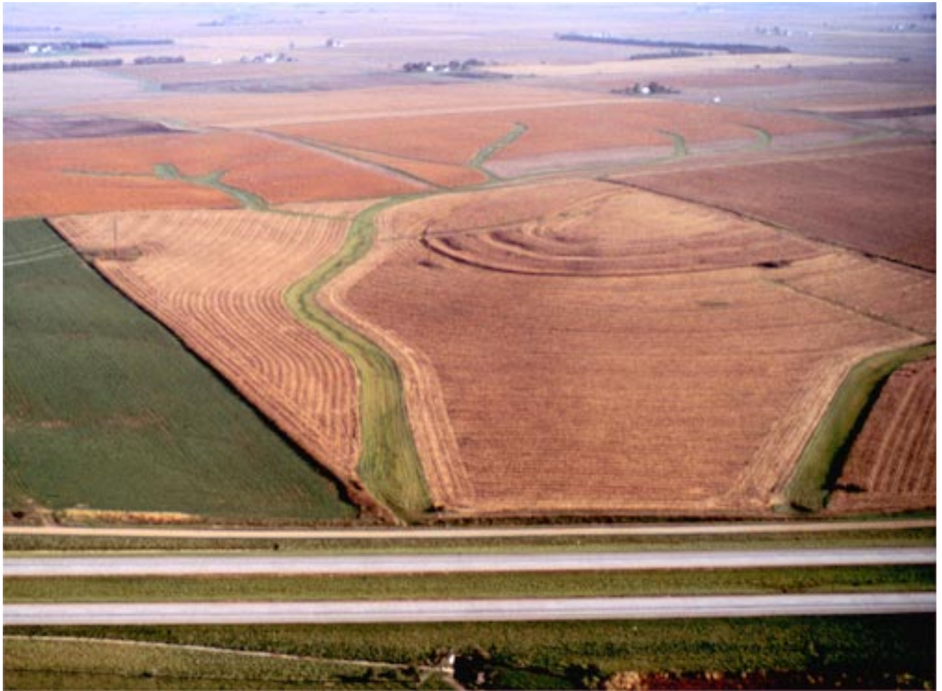
Figure 5.—A combination of grassed waterways and narrow-based terraces helps to prevent further erosion in an area of Wyanet silt loam, 5 to 10 percent slopes, eroded.
