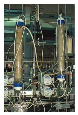
Figure 1. Two current biotrickling filters from which all biomass
