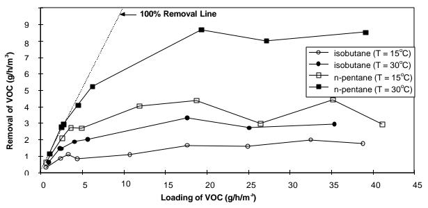
**Figure 3.** Removal Efficiencies in Trickle-bed Bioreactor. Removal efficiencies are highest as the residence time within the trickle-bed system increases. Of the two gases, n-pentane is preferentially removed. The solid line represents 100% removal. Data above were collected for low initial gas phase concentrations in the VOC feed. Higher removal rates are obtained when the initial gas phase concentration is raised.
