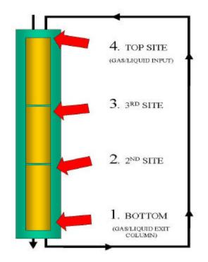
Figure 3. Simple diagram of the biotrickling filter showing sampling points for population and distribution assay
