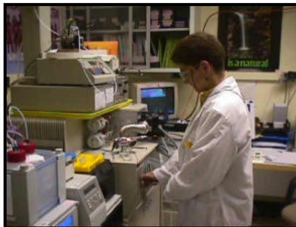
A Chemistry Investigator injects a rat plasma sample through the liquid chromatograph for analysis of estrogenic phytochemicals and metabolites using electrospray mass spectrometry.
