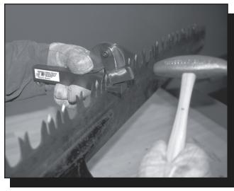
Figure 4—Setting the tooth with the crosscut saw tooth-setting tool.
