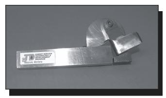
Figure 1—A crosscut saw tooth-setting tool. A hammer is used to
