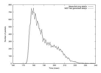
Figure 6: Real vs. NIST Net-synthesized delay distributions
