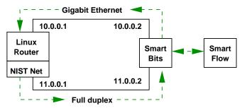
Figure 11: NIST Net testbed configuration
