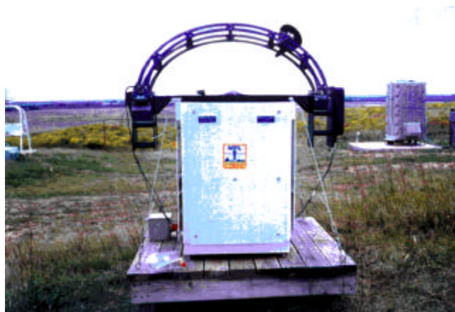
Figure 1. Day/night whole sky imager fielded at the SGP CART site. (For a color version of this figure, please see http://www.arm.gov/docs/documents/technical/conf_9803/shields-98.pdf .)
