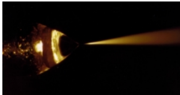
Figure 16 Typical electro spray jet in vacuum. The electro spray needle, liquid meniscus, and emitted spray are observed in this picture. The outside diameter of the tube is 0.3 mm.
