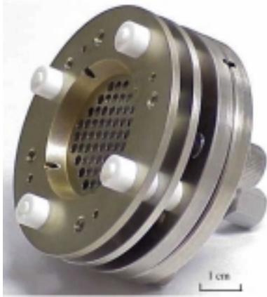
Figure 12 The 20- \mu N colloid thruster, which has 57 needles (nano droplet emitters), extractor grid, and an accelerator grid. The double grid is necessary to achieve the required thrust stability.
