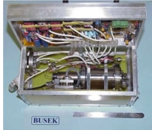
Figure 15 The 20- \mu N colloid thruster system during integration with the power-processing unit
