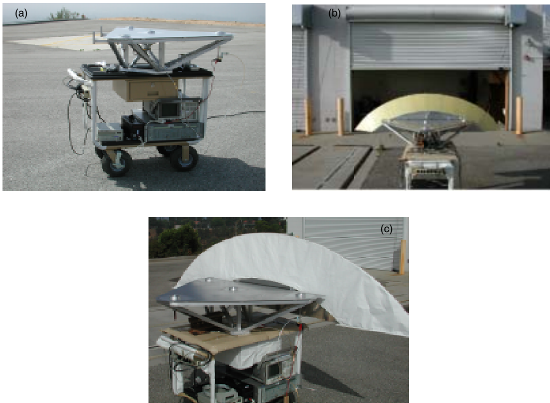
Fig. 2. Test setups for the isolation between transmitting and receiving antennas: (a) with no sunshade, (b) with the collector spacecraft sunshade, and (c) with the combiner spacecraft sunshade.
