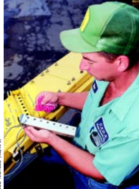
Dan Shirley, Beltsville Agricultural Research Center farm operations branch supervisor, inspects yield-monitoring sensors his crew installed on a silage harvester.
