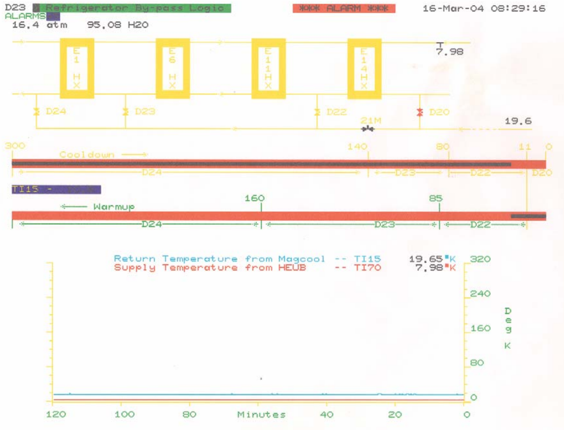
Figure 1 Display of control page D23 for cooldown control of HEUB refrigerator
