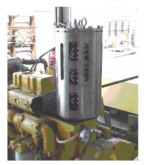
Figure 2. Alternator Test Rig
