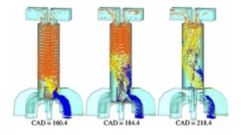
Figure 3. Calculated Stratified-Scavenging Flows
