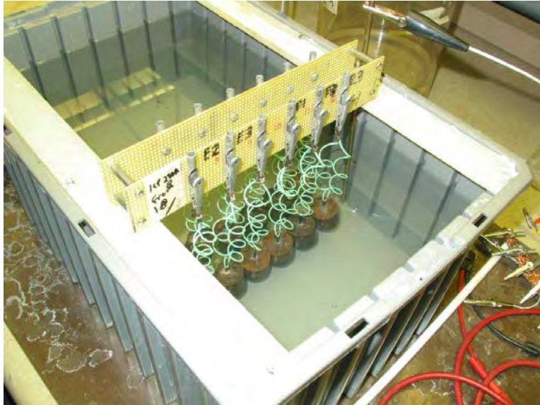
Figure B-2. CP (10-Times Static Wrapped) Test Specimens in Wet DWV Test
