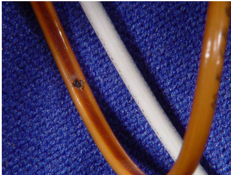
Figure 64. Unaged PV Wire (White) and Wire Aged for 570 Hours
