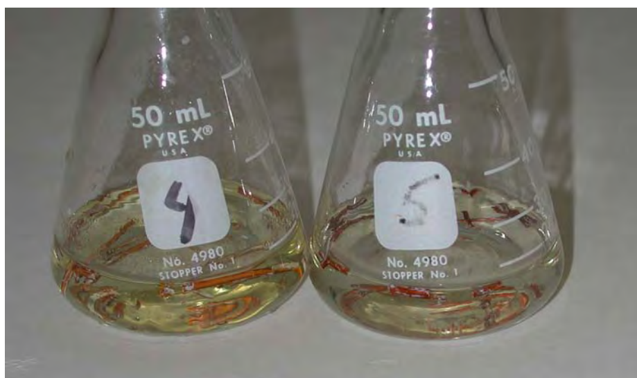
Figure B-13. Very Little Discoloration of CP Wire
