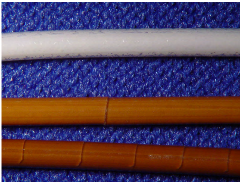
Figure 67. Unaged PV Wire (Top) and Aged Wires (Bottom) for 4200 and 5200 Hours
