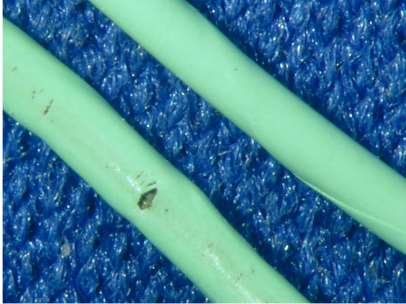
Figure 41. Unaged CP Wire (Right) and Aged Wire (Left), DWV Test
