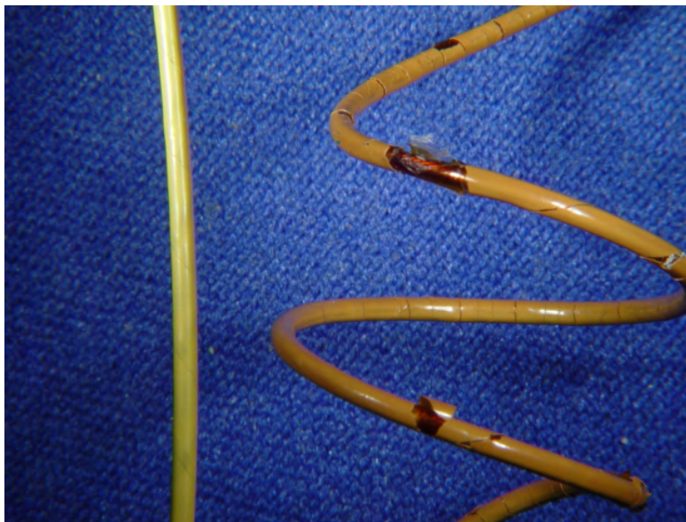
Figure 19. Unaged PI Wire (Left) and Aged Wire (180 Hours)
