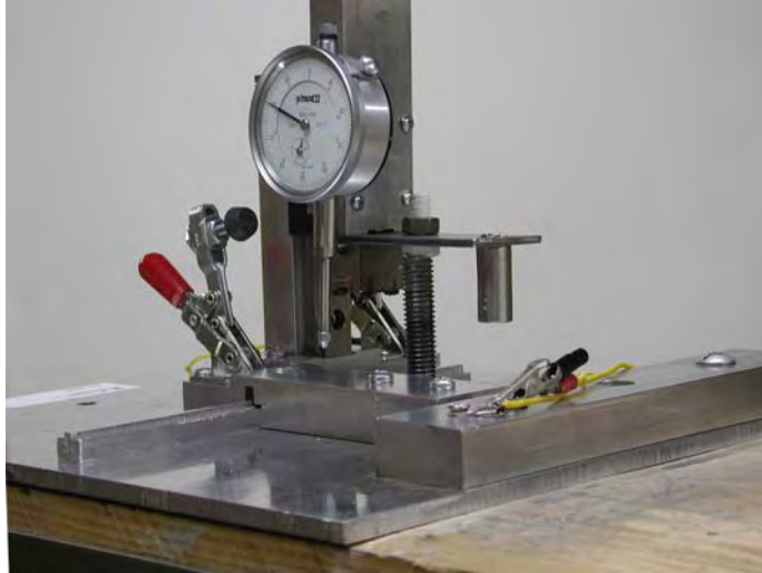
Figure G-34. The Static Cut-Through Apparatus Used to Test PI, CP, and PV Wire
