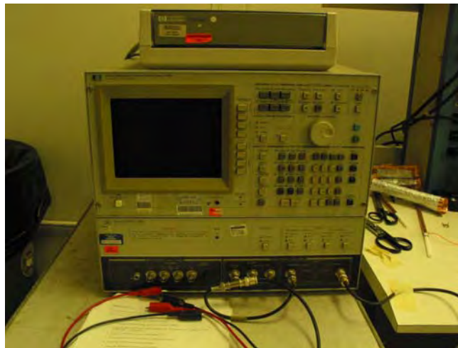
Figure G-21. Phase Angle Test Equipment
