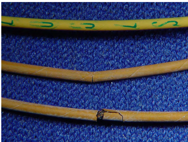
Figure 15. Progression of Insulation Damage, Aged at 300°C
