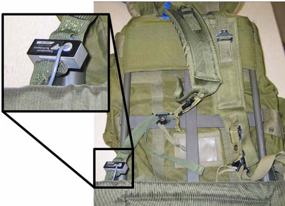
Figure 6: Instrumented backpack used to experimentally determine the loading in the straps.
