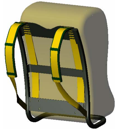
Figure 23: Schematic of the backpack with piezoelectric straps.
