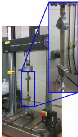
Figure 10: Experimental setup used to apply a controlled tension to the strap while the power output is measured.
