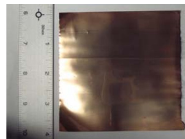
Figure 9: Piezo film transducer fabricated with self-assembled Metal Rubber surface electrodes.
