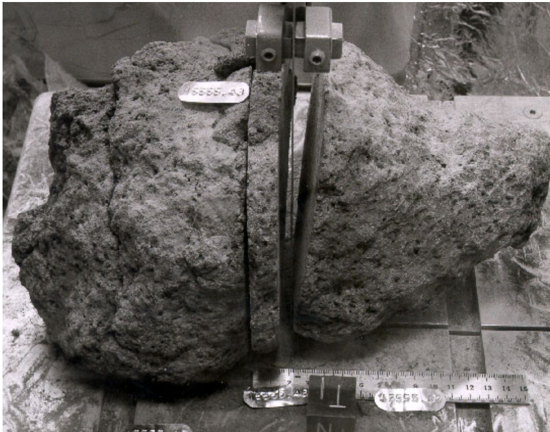
Figure 19: First saw cuts of 15555. Photo number S71-57110. Cube is 1 inch.
