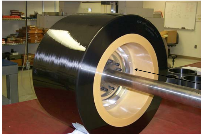
Interior view of 5-kWh rotor, showing circumferential crack near the hub
