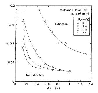
Fig. 5 Measured critical agent mole fraction at suppression as a function of agent injection period.
