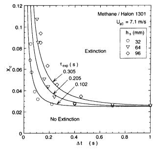
Fig. 6 Measured critical agent mole fraction at suppression and theoretical curves as a function of agent injection period.
