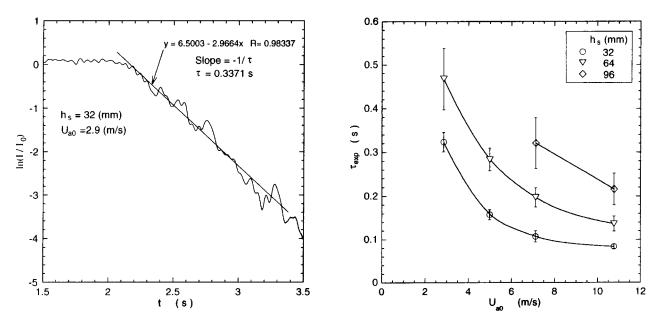
Fig. 2 Sodium D-line emission intensity trace.
