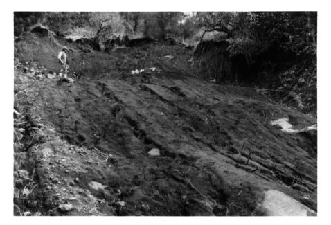
Figure 6 Source area and upper runout path typical for small debris flows, Kuliouou Valley, Oahu, Hawaii, January 1, 1988. The length (42 m) and width (16 m) of the source area greatly exceed the thickness (1-2 m) of the failed soil mass, indicating that a one-dimensional infinite-slope analysis might be appropriate. The average slope angle is  $32^{\circ}$ .
