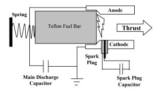
Figure 2. PPT Diagram
