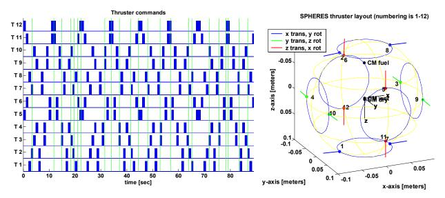
Since PADS was non-operational for the KC flights, the 12 SPHERES thrusters were commanded in repeating, 24seconds long, open loop sequence as shown here. There were always either 0 or 2 thrusters firing to minimize the effect of uncertainty in thrust reduction with multiple thrusters firing. This sequence fires forward then backward on each of the 3 rotational axes, then the 3 translational axes, then all that backwards. Each pulse is 0.8 seconds long,
