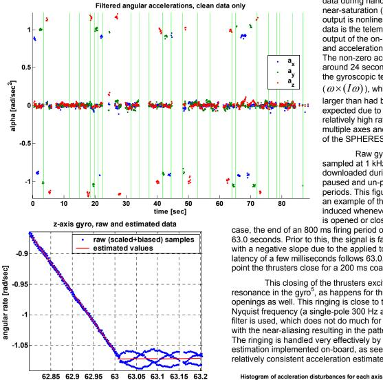
time [sec] previous plot. The segments defined by the onboard-estimated rates and accelerations are overlaid on the raw gyro data to demonstrate the estimator's ability to filter out the gyro ringing while providing accurate and high bandwidth estimation. The acceleration estimates (slopes of the red lines in the plot) before and after thruster closing are:
