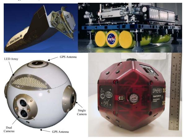
Figure 1: Four of the vehicles successfully tested in simulation. Clockwise from upper left: X-38 v. 201 with de-orbit propulsion stage; NASA Ames S4 air bearing vehicle; MIT SPHERES; JSC Mini AERCam. Hardware implementation and testing is currently underway on the S4 and SPHERES.
