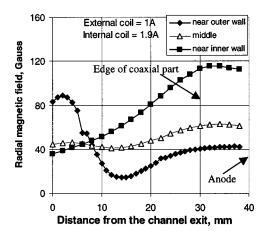
FIG. 4. Radial magnetic field in thruster channel.
