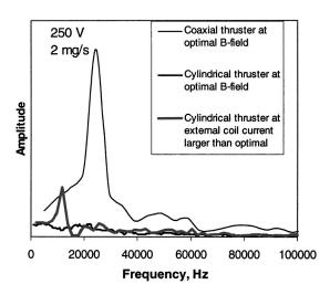
FIG. 9. Spectrum of oscillations in the cylindrical and coaxial Hall thrusters, at a discharge voltage of 250 V and mass flow rate of 2 mg/s.
