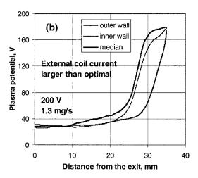
FIG. 10. Plasma potential profiles measured at different magnetic fields: (a) optimal, corresponding to the minimum discharge current; (b) above optimal.
