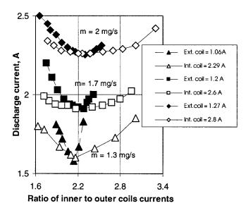
FIG. 8. Discharge current for different magnetic configurations. Current variations in the electromagnet coils, external and internal, change both the magnetic field magnitude and its distribution in the channel.
