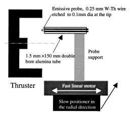
FIG. 5. Schematic of the fast emissive probe setup.
