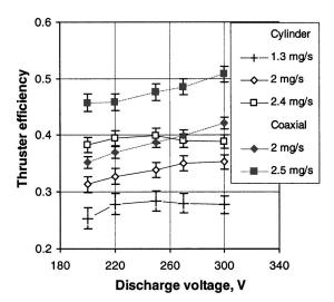
FIG. 14. Thruster efficiency of the cylindrical thruster. Note comparison to the coaxial Hall thruster. The results do not include the cathode flow rate of about  $0.2\ \text{mg/s}$ .
