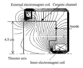
FIG. 3. Magnetic field simulations of the laboratory thruster.
