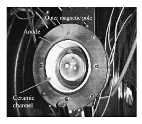
FIG. 2. A 9 cm laboratory cylindrical Hall thruster.
