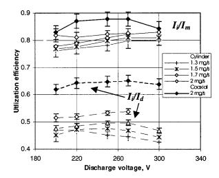
FIG. 13. Propellant utilization,  $I_i/I_d$ , and current utilization,  $I_i/I_d$  of the cylindrical thruster. Note comparison to the coaxial Hall thruster. The propellant utilization does not include the cathode flow rate of about 0.2 mg/s.
