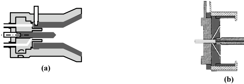
FIGURE 2. Schematics of a.) MYII Thruster (Tahara, 1985) and b.) Princeton Benchmark Thruster (Choueiri, 1998b) (Drawings are not to scale).
