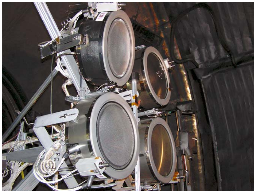
Figure 2. Three + one NEXT array; array installed into VF6 test facility at NASA GRC. EM1 thruster is gimbaled.
