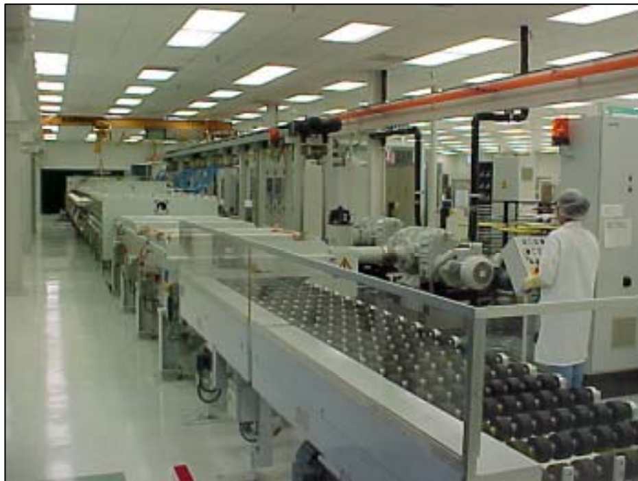
Figure 24. New high throughput base electrode and precursor sputtering equipment.
