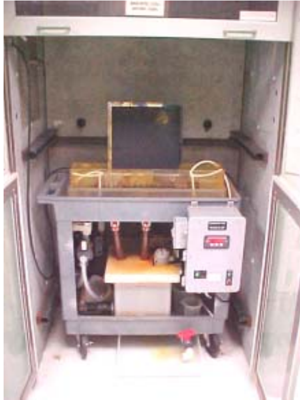
Figure 33. Test fixture etching based edge deletion.
