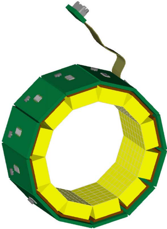
Fig. 4. Block detectors form a ring connected with a flexible cable that serves as bus for transmitting serial data of the ring and receiving power and control signals.
