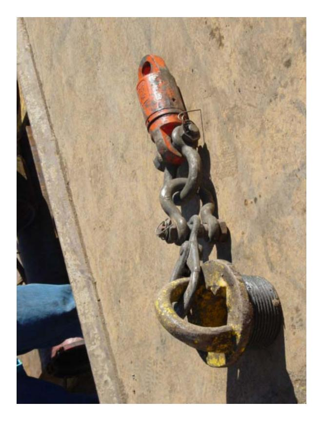
Photo of Lifting Sub that Replaced the Nylon Strap
