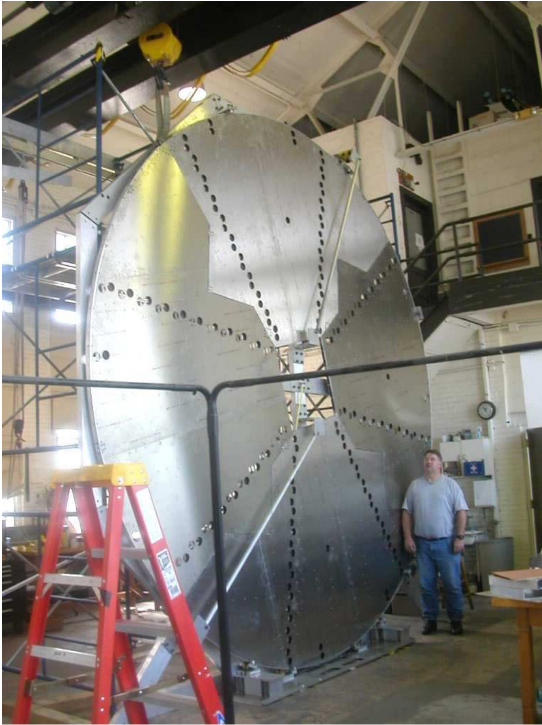
Figure 7.18: A full sized mockup of a muon detector mounting wheel. Built and installed at the University of Illinois.
