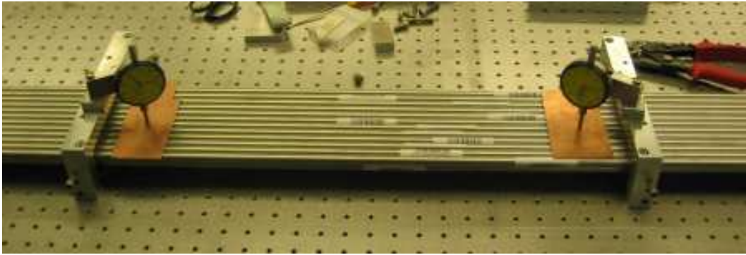
Figure 7.23: Test rig for looking at wire stability at high voltage for one of our long (6 ft.) planks.
