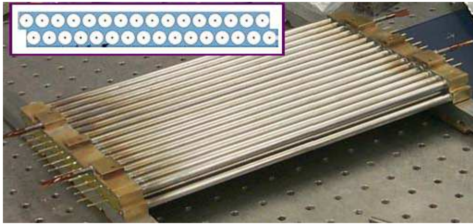
Figure 7.2: The basic building block of the muon system (plank). The inset shows an end view of the plank, and demonstrates the “picket fence” geometry of the proportional tubes. The gold colored pieces at each end of the plank are the brass gas manifolds. Visible at the end is the circuit board soldered around the edge to the brass piece.
