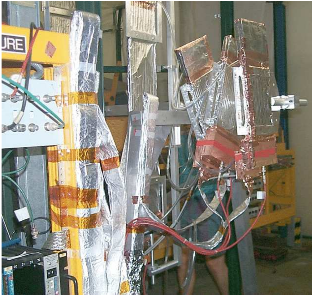
Figure 7.11: The BTeV muon system setup for the 1999 test beam run. Five planks are visible in this photograph. Noise problems required shielding with aluminum foil and copper tape.
