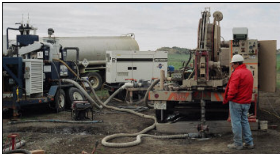
LANL microdrilling at the RMOTC-operated Teapot Dome Field at NPR No. 3. The microdrilling rig includes the coiled tubing drilling unit on the right, mud cleaning system on the left, and the RMOTC drilling-water truck in the center.
