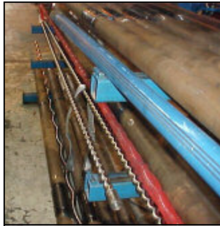
Slimhole electric submersible motor.
