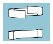
• Ideal for smaller head screws, such as socket head cap screws, where clearance may be a problem. Greater thickness compensates for smaller outside diameter allowing performance similar to a regular section.
