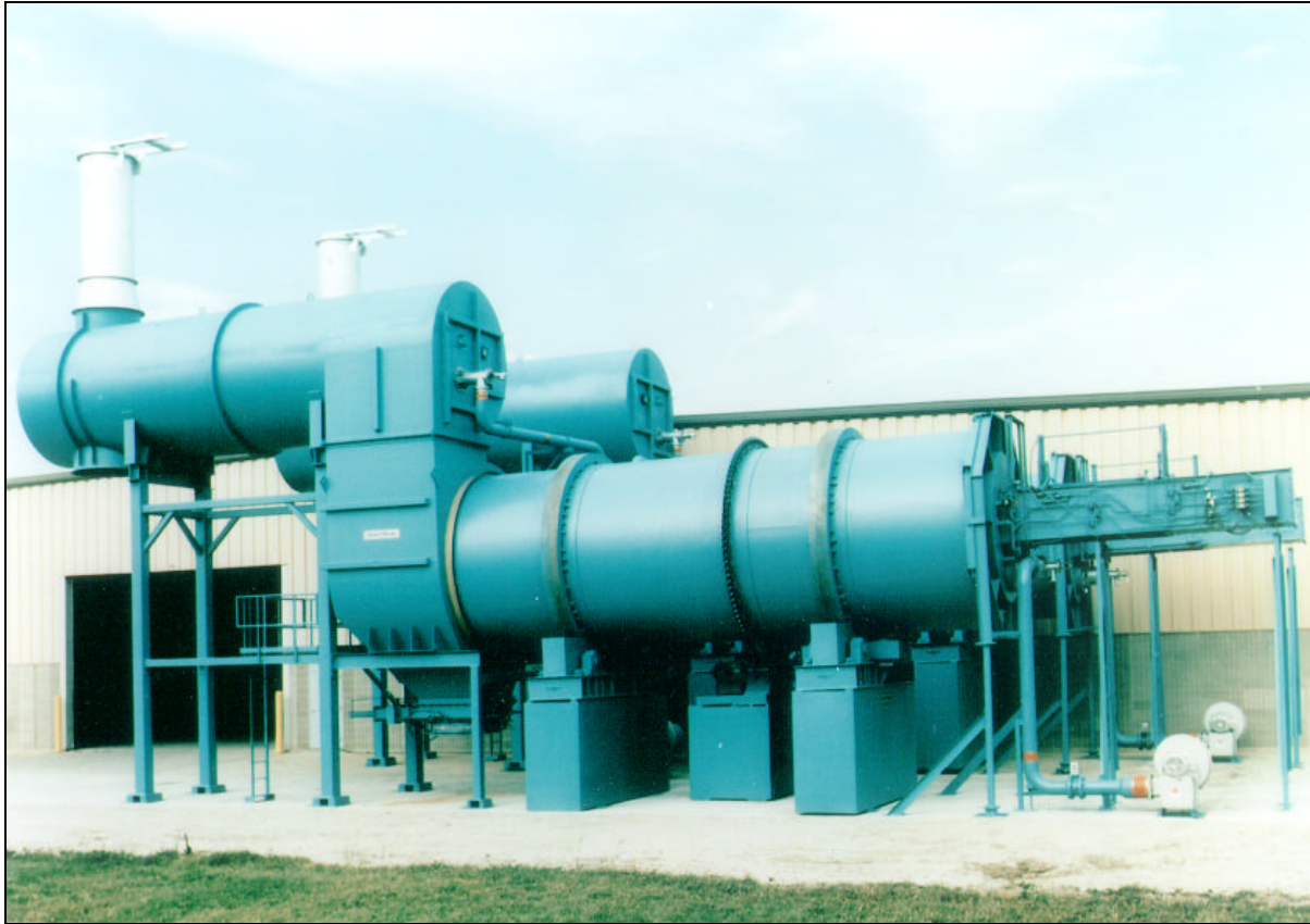
Figure 2. Andersen 2000 Rotary Kiln Melter for the Cement-Lock™ Demonstration Project (Two kilns shown)
