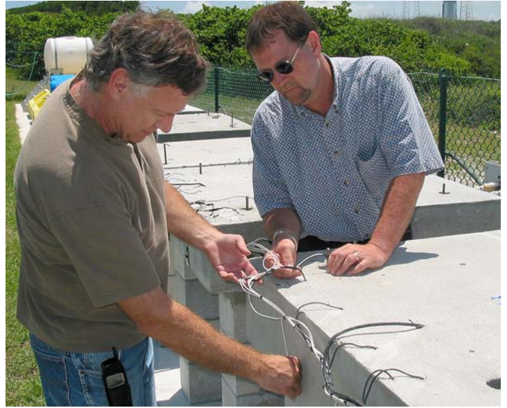
Joe Curran (left), corrosion engineer with Dynacs Engineering Co. Inc. and Louis MacDowell, NASA Testbeds manager, inspect reinforced concrete being tested at the Corrosion Technology Testbed.
