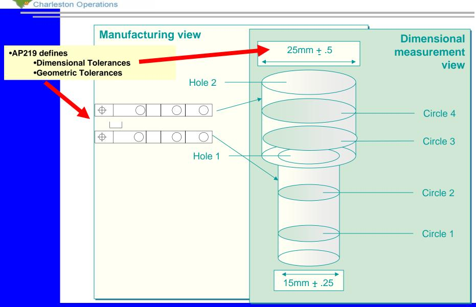
Instances: Counterbore\_hole measurement Northrop Grumman
