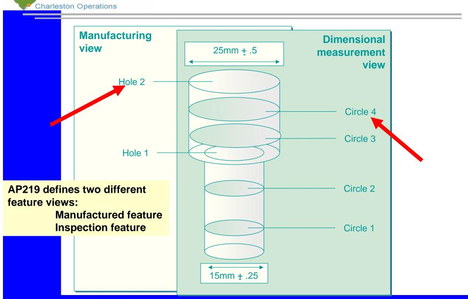
Instances: Counterbore\_hole measurement Northrop Grumman
