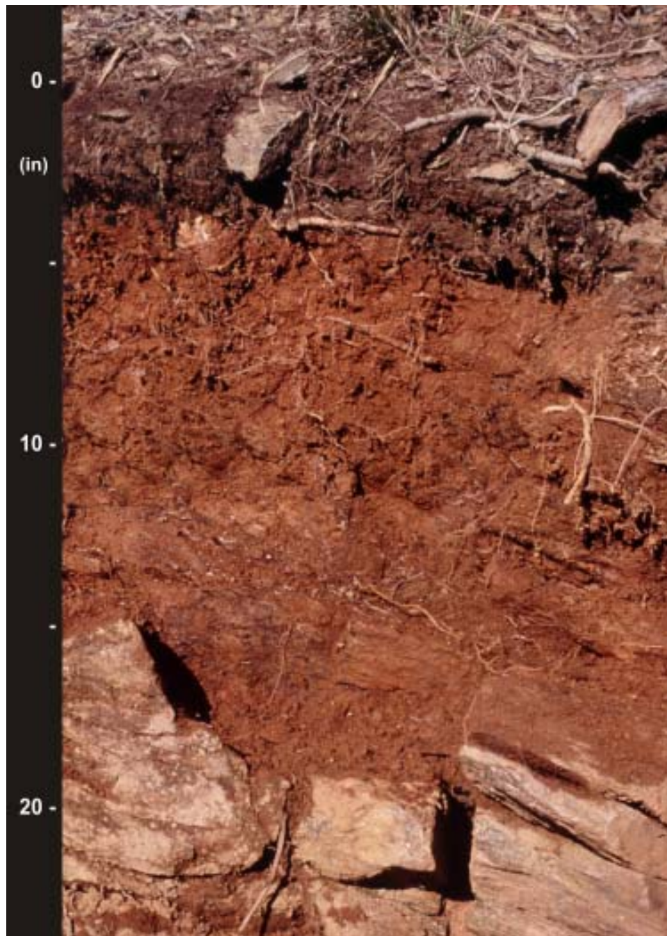
Figure 22. —A profile of Cleveland gravelly fine sandy loam in an area of Cleveland-Rock outcrop-Peaks complex, windswept, 10 to 45 percent slopes, very bouldery.
