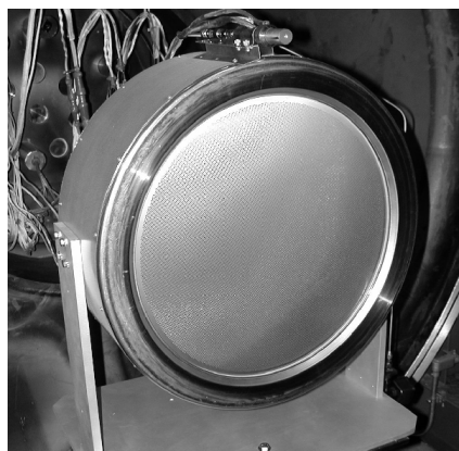
Fig. 3. Photograph of the 40 cm NEXT laboratory model ion engine with ion optics installed.
