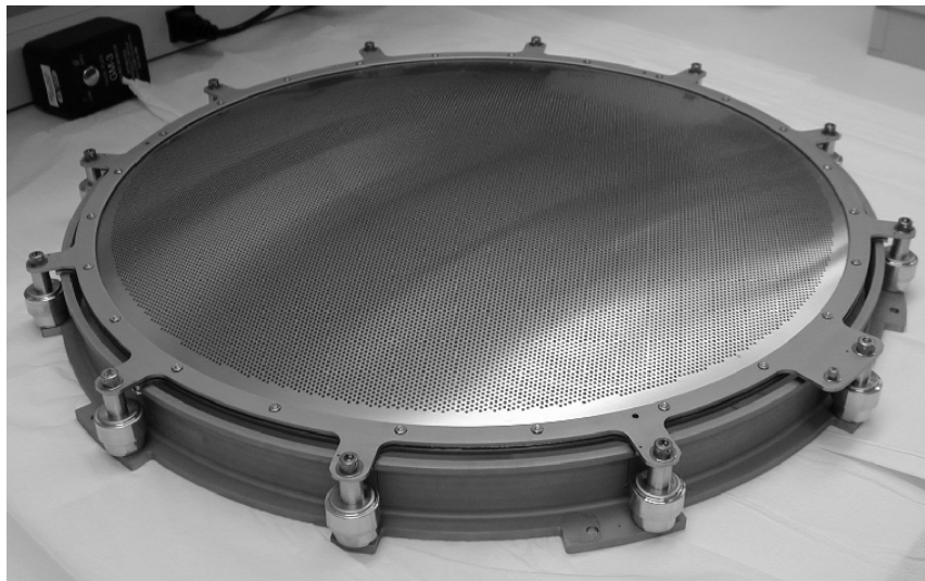
Fig. 2. Photograph of 40 cm ion optics installed onto a 40 cm engineering model mounting assembly.
