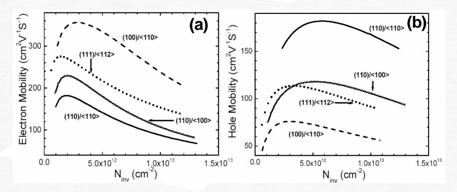
Orientation effect on the (a) effective electron mobility, (b) effective hole mobility as a function of inversion carrier density. Electron mobility is the highest on the (100) surface while the hole mobility on the (110) surface is more than 2.5 times higher than that on the (100) surface. Reproduced with the permission of M. leong et al., (IBM) and The Electrochemical Society, Inc.
