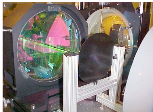
FIGURE 6. Test end of the IR 2 setup for TTV measurements of 300 mm wafers. The picture shows the collimator lens together with a silicon wafer and a return flat.
